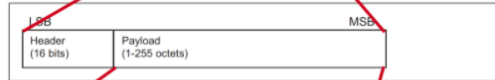
Figure 2.4: Advertising physical channel PDU
