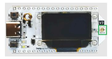
Attach the antenna cable to the U.FL connector on the Heltec WiFi LoRa 32 v3 board.
