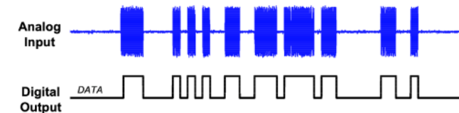
Figure 2: Example OOK signal at the input to the receiver and its corresponding demodulated output.
