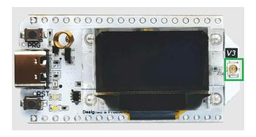
Attach the antenna cable to the U.FL connector on the Heltec WiFi LoRa 32 v3 board.
