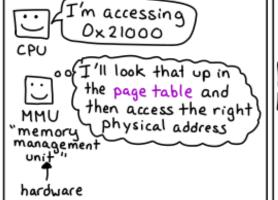
every time you switch which process is running, Linux needs to switch the page table
