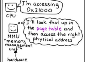
every time you switch which process is running, Linux needs to switch the page table
