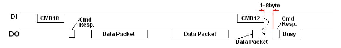
SD card delays can be significant
