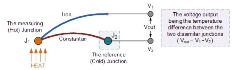
Thermocouple generates a voltage based on temperature
