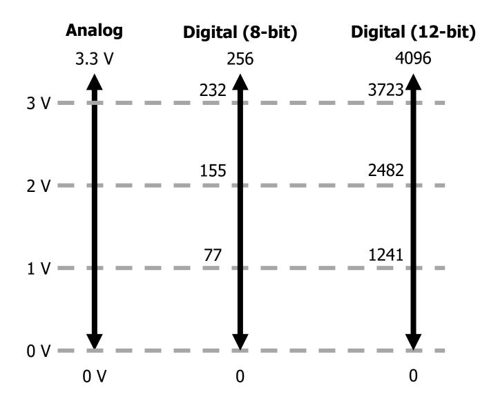
$$Value = \frac{V_{IN}}{V_{REF}} * (2^{Resolution})$$
