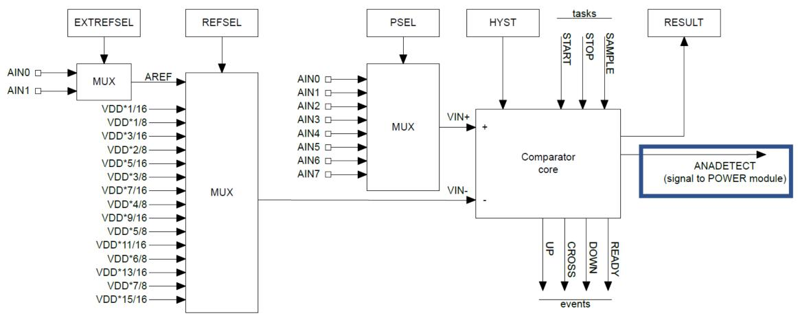
• Can be used for low-power wakeup of microcontroller
