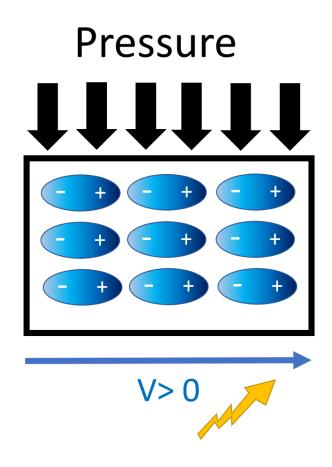
Alternative to resistive sensors. But, a voltage is still the output
