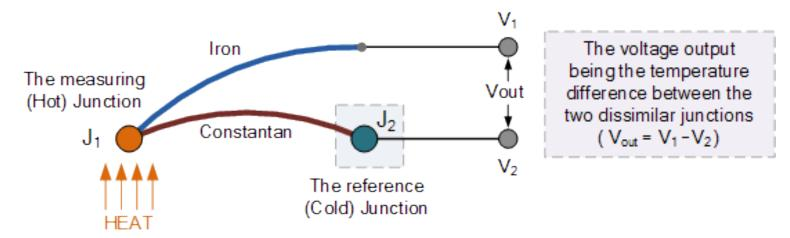
Thermocouple generates a voltage based on temperature
