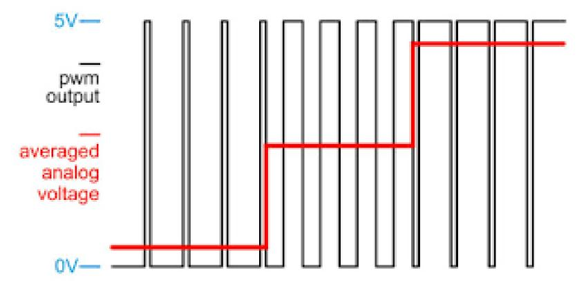
• PWM period should be much faster than the desired analog signal
