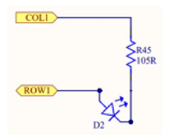
COL1-5 are usually nRF52 outputs that are used to sink current to selectively illuminate LEDs. Note that for light sensing the LEDs must be reverse-biased. COL1, 3 & 5 are connected to nRF52 ADC-capable pins but light sensing is currently digital.
